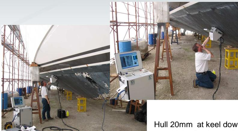
Hull 20mm at keel down to 12.5
