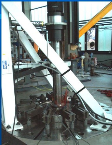
Total view of the axle prepared for fatigue test on the Sincotec machine
