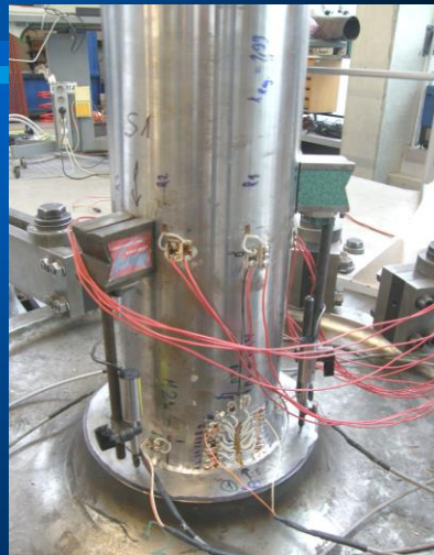
LVDT extensometers measuring displacement between axle and wheel
