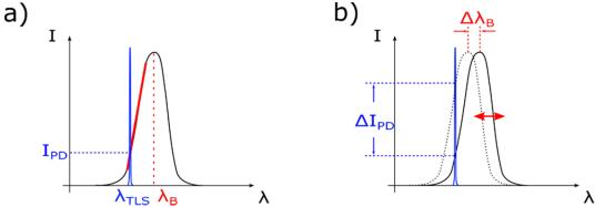
**Fig. 2.** Edge filter detection method working principle: (a) Tunable laser wavelength (blue line spectrum,  $\lambda_{TLS}$ ) is set within the linear slope of the FBG spectrum (red line). (b) An incoming acoustic wave will cause the FBG to vibrate resulting in Bragg wavelength shifts and in turn changes in the intensity of the back-reflected signal.
