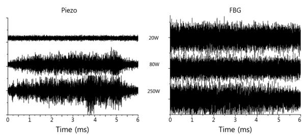
**Fig. 4.** Response of piezoelectric (left) and edge filter FBG sensor to the acoustic wave generated for 20, 80 and 250 W average power laser weld in TiAl4V6 plates (Titanium Grade 5).
