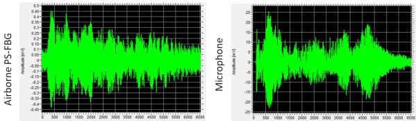
**Fig. 6.** Airborne PSFBG waveform versus a microphone during a 5 ms duration laser welding experiment. Time scale in the *x*-axis is in  $\mu$ s.
