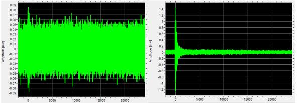
**Fig. 5.** Response of uniform FBG (left) and PSFBG (right) to the AE of a pencil lead break. An 11dB increase in the SNR is observed by using the PSFBG. Time scale in *x*-axis is in µs.
