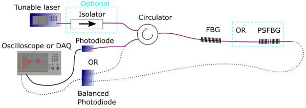
**Fig. 1.** Edge filter method setup for the detection of AE using FBGs or phase-shifted FBGs (PSFBGs). Dotted line connections refer to the case of using a balanced photodiode.
