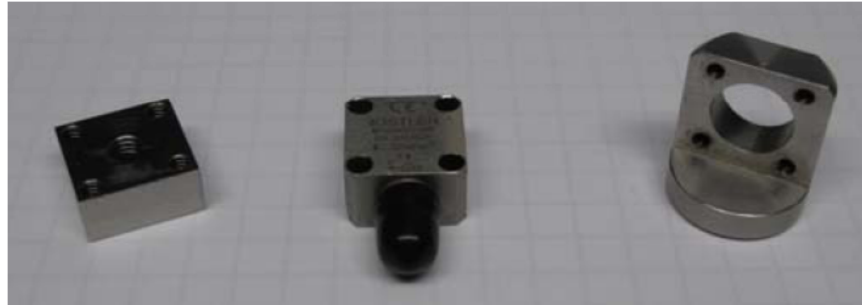
Figure 3. Mounting adapters used to calibrate the z-axis (left) and the x- and y-axes (right) of a triaxial accelerometer Kistler type 8793A500 (center).
