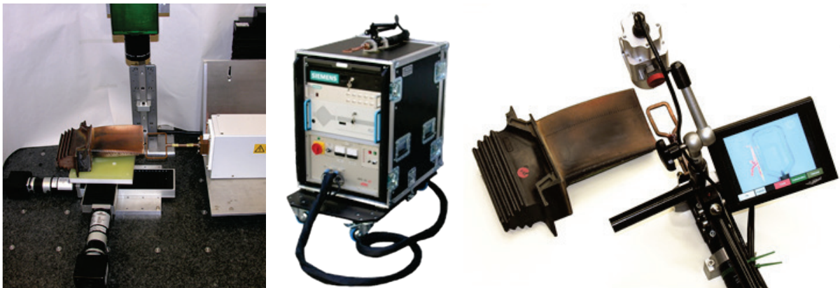
Fig. 4: Left: Stationary lab induction thermography system (top: infrared camera, right: auxiliary device of the induction generator); Right: Mobile and handheld induction thermography system (left: portable rack including the generator and all the necessary equipment, right: auxiliary device with a small infrared camera and a touch screen display mounted to it) [2].
