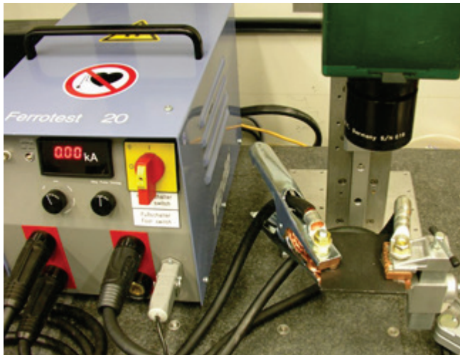
Fig. 6: Conduction thermography system and resulting image calculated by pulse-phase analysis. The “crack” (several holes drilled into the component next to each other) in the center of the test component is clearly visible [2].
