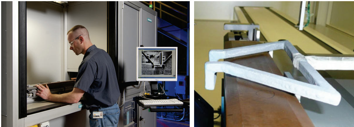
Fig. 5: Left: View of the automated induction thermography inspection system from the outside Right: Component under test and induction coil [4].
